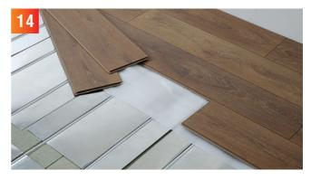
Both engineered and laminate can be installed directly on the heat transfer plates using a low TOG underlay. A minimum of 8mm engineered or laminate must be used.
