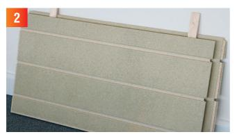
Before installation, the moisture content of the ProFloor boards should be stabilised close to the conditions of use. The boards should be stabilized for 5-7 days, depending on the initial moisture content. The boards should be separated with battens whilst being stabilised.
